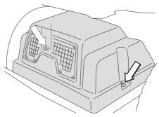
2 Rider 13 C and Rider 16 C Check that there is oil in the transmission's oil tank. Fill if necessary with engine oil SAE 10W/30 (class SF–CC).
